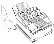
2. Insert the power cable into the power inlet socket located on the back of the fax machine.
